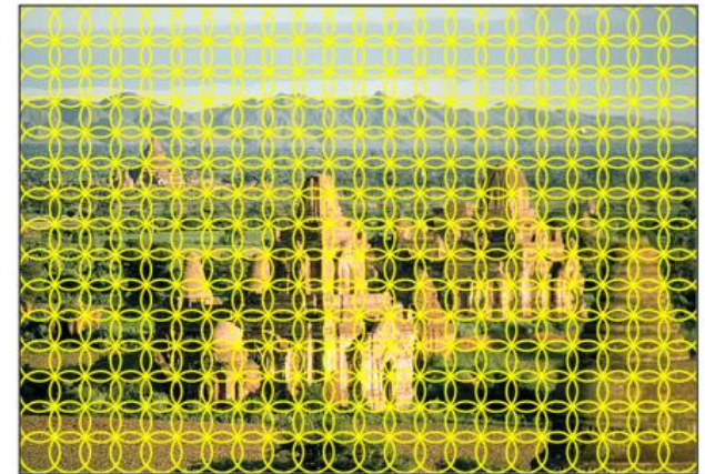
SIFT descriptors of 16x16 patches sampled on a regular grid, quantized to form visual vocabulary (size 200, 400)
