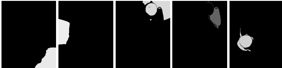
Figure 16.15. Five of the segments obtained by segmenting the image of vegetables with a k -means segmenter that uses position as part of the feature vector describing a pixel, now using 20 segments rather than 11. Note that the large background regions that should be coherent has been broken up because points got too far from the center. The individual peppers are now better separated, but the red cabbage is still broken up because there is no texture measure.
