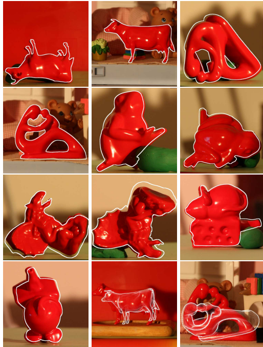
Figure 4. Examples of the pose estimation results on real indoor images. The white contour corresponds to the occluding contour of the object in the estimated pose. The two images in the bottom right corner show the failure cases.
