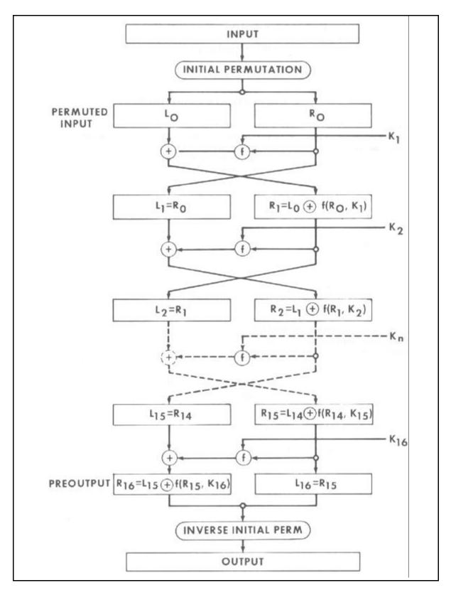
Figure 1. Enciphering computation.
