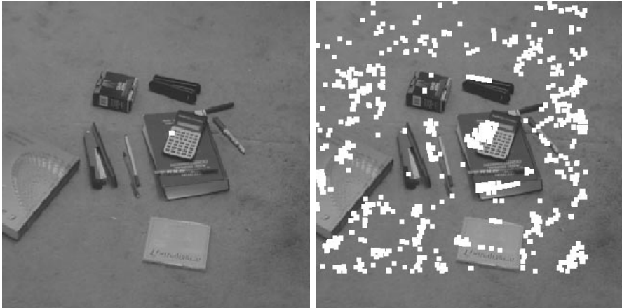
Fig. 7. Detection of pocket calculator, anti-face method (left), and eigenface method with a face space of dimension eight (right).
