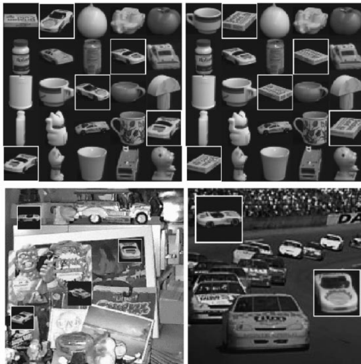
Fig. 12. Top: Detection of 3D objects from the COIL database: A toy car is sought in the left image; a chewing gum bar in the right. Bottom: Detection of 3D objects from the COIL database: A toy car is detected in general background setting. The car model in the center (left image) is different than the one being sought. Detection is marked by a white square around the detected image region. The average number of detectors per pixel was 1.31.
